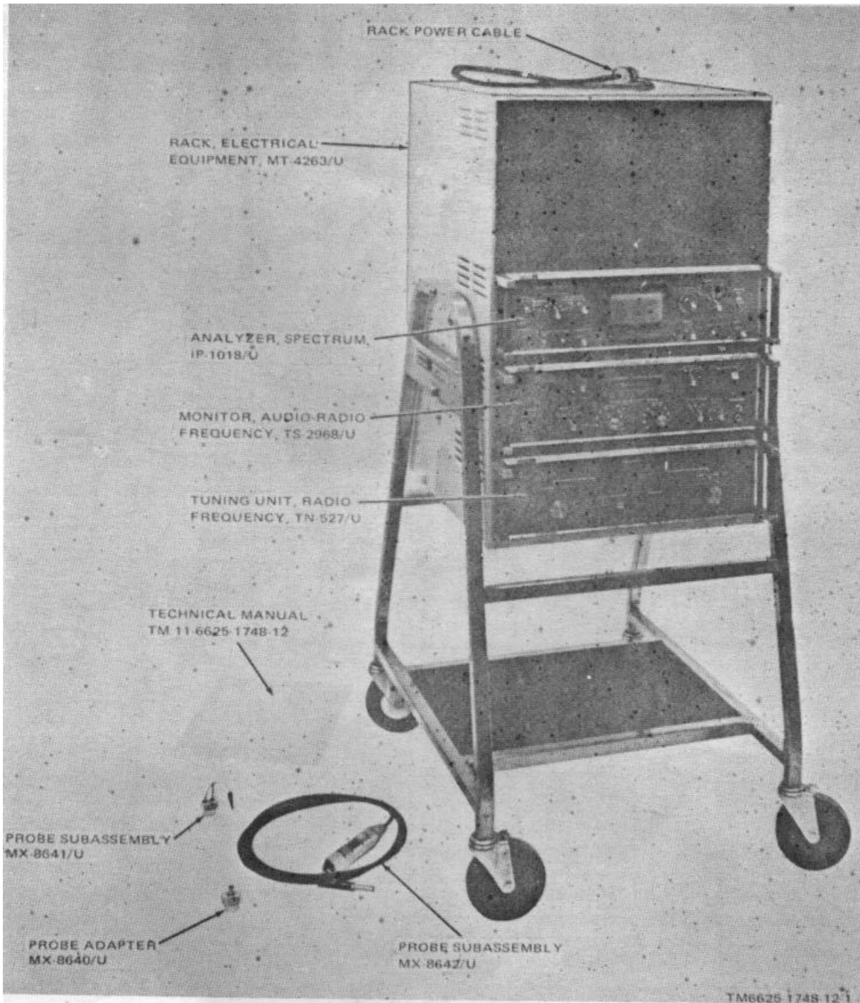
Figure 1-1. Test Set, Radio AN/USM-306(V)1.
